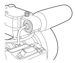
2 Connect the microphone connecting cable to the unit's MIC IN jack.
